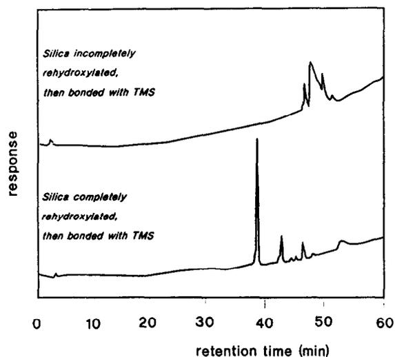
Fig. 5. Effect of bonded phase hydrolysis on the chromatography of a basic peptide (melittin). Top, freshly prepared TMS phase on fully rehydroxylated Zorbax PSM 60; bottom, the same separation after 50% hydrolysis of the TMS phase (1 month of operation). Mobile phase: 0 to 100% acetonitrile in 0.1% trifluoroacetic acid over 80 min, 1 ml/min at 50°C. Figure reproduced from ref. 52.
