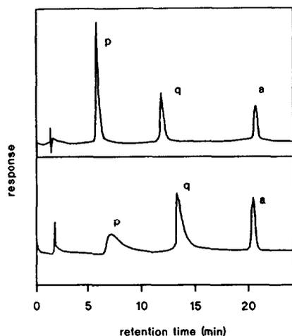
Fig. 2. Comparison of the chromatography of chelating species on silicas with different metal contents. Top: Kromasil C18; bottom: Develosil C18. Peaks: p = purpurin; q = quinazarin; a = amybenzene. Mobile phase: 75% methanol–0.05 M phosphate buffer, pH 3. Figure reproduced from ref. 31.
