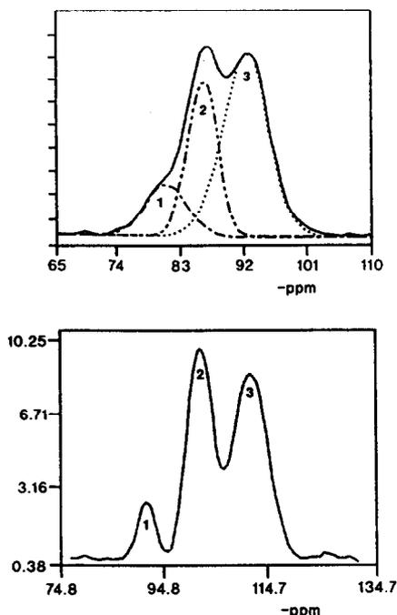
Fig. 1. Comparison of  $^{29}\text{Si}$  cross-polarised magic angle spinning NMR spectra. Top: dry silica. Bottom: silica saturated with water vapour. Peaks: 1 = geminal silanols; 2 = isolated silanols; 3 = structural siloxane bridges. Figure reproduced from refs. 11 and 20.
