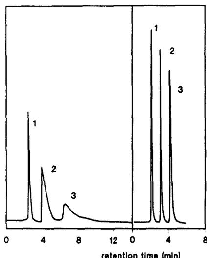
Fig. 4. Illustration of the beneficial effects of end capping. Left, uncapped C18 silica, prepared from a silica containing moderate metal concentrations; right, separation performed on the same material after end capping. Samples and conditions as in Fig. 3. Figure reproduced from ref. 30.
