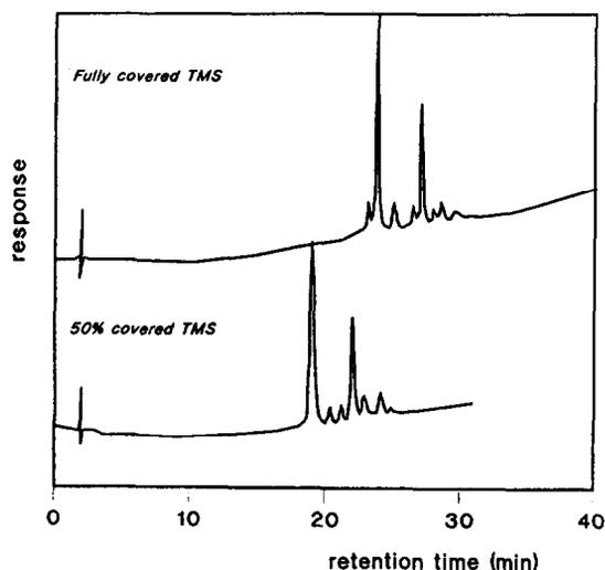
Fig. 6. Effect of the degree of rehydroxylation of the silica upon the separation of lysozyme, melittin and ovalbumin. Top, TMS phase prepared from inadequately rehydroxylated silica; bottom, TMS phase prepared from fully rehydroxylated silica. Other conditions as in Fig. 5. Figure reproduced from ref. 52.
