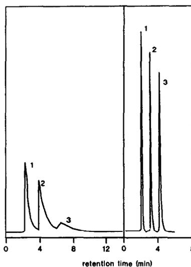
Fig. 3. Comparison of the effects of amines content upon the reversed-phase chromatography of amines on capped ODS packings. Left, silica containing a high concentration of metals; right, silica prepared from purified sodium silicate. Peaks: 1 = aniline; 2 = N-methylaniline; 3 = N,N-diethylaniline. Mobile phase: 5% methanol–0.02 M phosphate buffer, pH 2.7. Figure reproduced from ref. 30.
